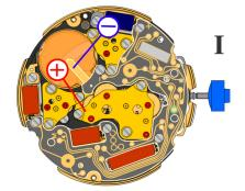
Setting stem in position I, calendar not in gear, 60 s measuring interval for rate and consumption:
