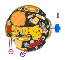
Coil resistance M1 1.90 k $\Omega$  .. 2.10 k $\Omega$
