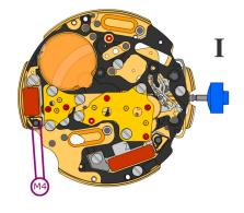
Signal generator (4.9 ms, 8 Hz):
