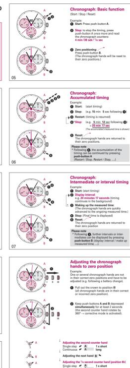
Adjusting the 1/10 second counter hand (position 6h) Single step A 1 x short Continuous A long
