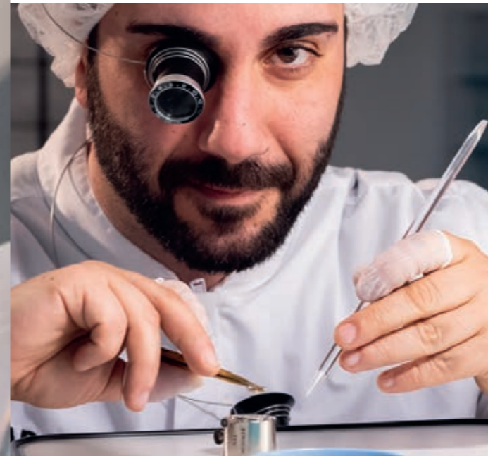
Stefano Diaferio, rhabilleur, is responsible for the fine adjustment of the assembled mechanical watch movements.
